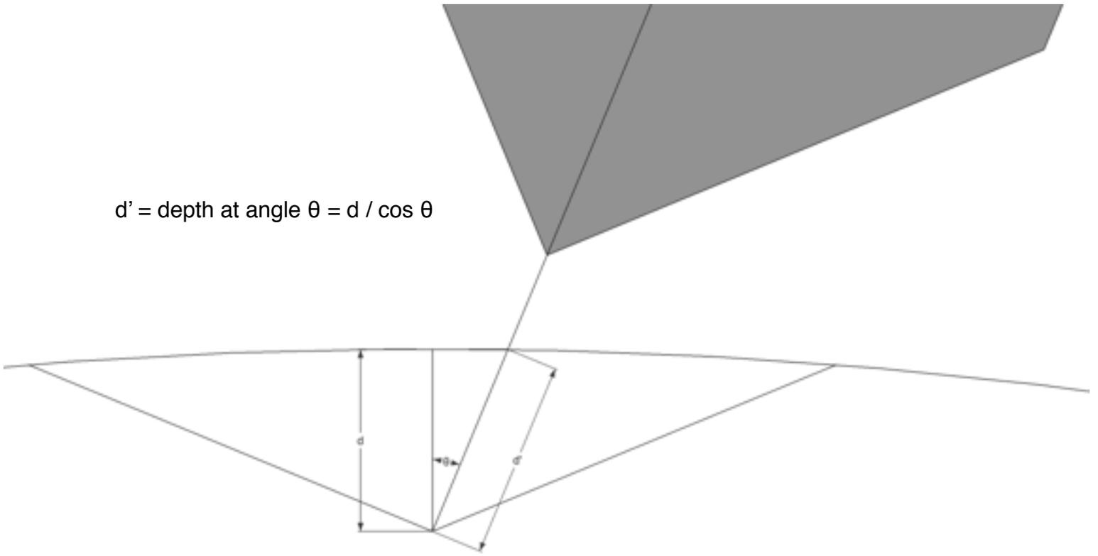
$D = \text{depth of cut for a smooth bead} = R - \sqrt{R^2 - Rc^2}$
