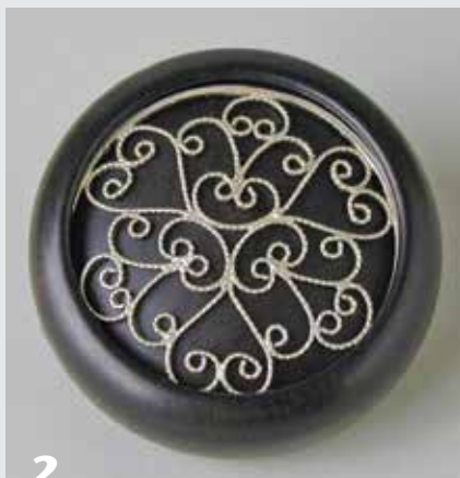
2 The wood lid expanded after exposure to high humidity, allowing the silver ring's edge to become visible.
