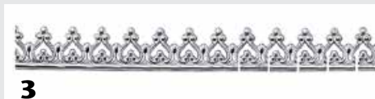
Sterling silver gallery wire shown without and with small saw cuts (left and right sides, respectively). This step is key to adding flexibility to a metal accent ring.
