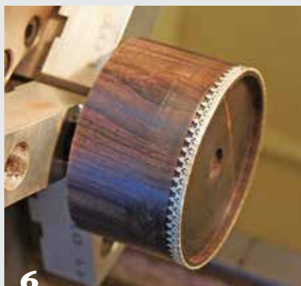
6 The silver band inset in a recess cut on the metal lathe.
