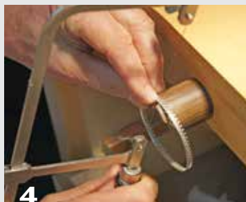
4 Sawing cuts at 1/8" (3mm) intervals with a jeweler's saw.
