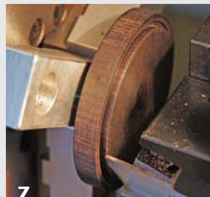
7 Cutting the groove in the retaining ring on the metal lathe. When the retaining ring is installed, this groove conceals the small cuts in the silver ring, allowing only the decorative filigree to show.
