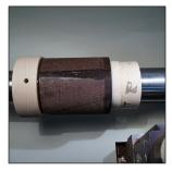
Cut the exterior off from the mounting block and turn the exterior to its final dimension (0.030" thick). Trim off the end to reveal the inner layers. When cutting the pattern, don't cut to the full thickness all at once. Do this in multiple passes.
