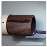
Get as close a fit as possible with the inner core.
