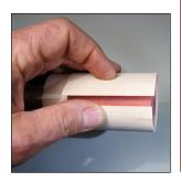
When dry, soak the veneer with CA glue and dry with accelerator. Turn the veneer down to the desired thickness (0.020") and trim the end of the cylinder.
