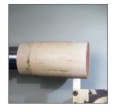
Square off the end of the exterior wood cylinder and drill the interior with a Forstner bit to a size slightly smaller than the final dimension. Drill a 1/4" hole through the bottom to connect with the vent hole. Using a boring bar, enlarge the interior to the final size.
