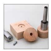
Attach the wood for the inner core on one MT2 arbor and mount the wood for the outer layer on a second MT2 arbor. Drill a hole in the scrap mounting block of the outer wood that goes through to the recess for the head of the mounting screw. This
