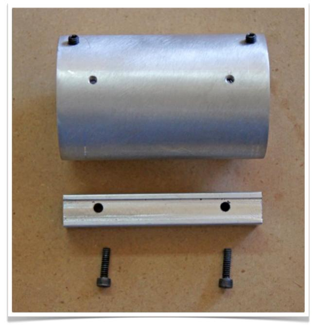
Pre-load on the bearings can be handled several ways. You can gradually trim the internal spacer to a point where tightening the end nut gives you the pre-load. If you take off too much, then you can add shims at the end of the internal spacer. Alternately, you can set the pre-load with the end nut in which case you will need a second locking nut (and you'll have to have a key between the pulley and the shaft or a set screw in the pulley).
