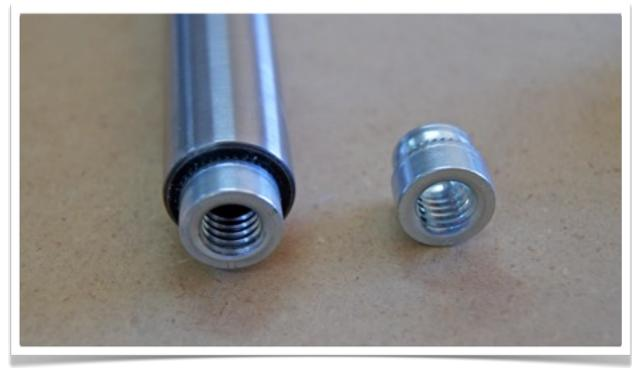
Then I made a pulley that mounted on the threaded insert so that I can use my overhead drive to power the drill frame. I lapped the
