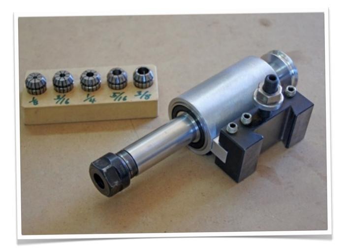
This article describes the construction of a precision drill frame (which can be used for an eccentric cutter) made from an ER16 extension chuck.
