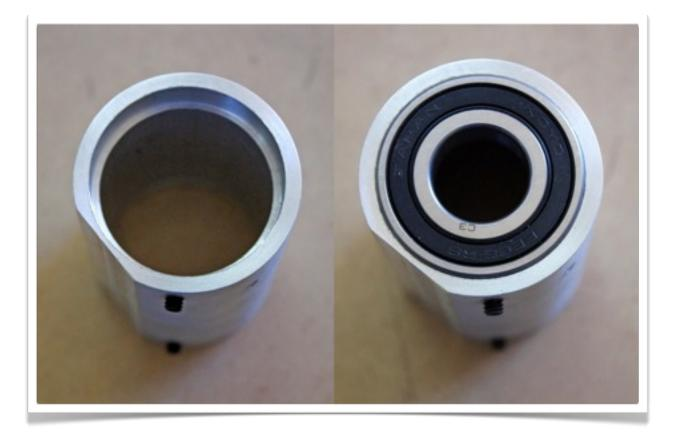
To mount the unit in the quick-change tool post, I used a piece of 1/2" x 5/8" 6061 Aluminum. On the edge, I milled a slot so that it would give me a stable fit to the outside of the round pipe and attached with 2 screws:
