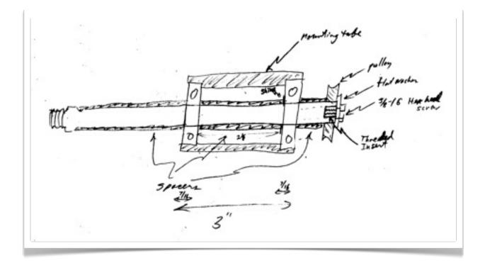
First, I press fit a threaded insert into the end of the ER16 extension (McMaster Carr #95185A330).
