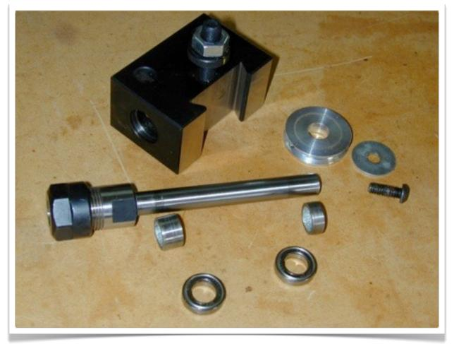
The screw on the end of the ER16 collet chuck shank is used to adjust the preload on the bearings. Tighten it until you feel some slight increase in the rotational resistance, then back off a bit. Secure it with Loctite.
