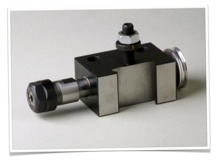
This article describes the construction of a precision drill frame (which can be used for drills, mills, or an eccentric cutter) made from an ER16 extension chuck. This is the 3rd generation drill frame I've made based on suggestions from John Alexander.
