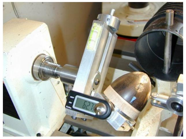
The bubble on the side of the frame is to let me accurately set the zero for the spindle rotation. Go to the Dollar Store and pick up a \$1 plastic level. Take it apart and you'll have 3 of these little bubbles that you can attach to any fixture with hot melt glue (thanks to Dewey Garrett for that tip).
