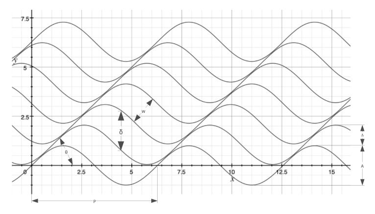
For a fixed cutter (used when cutting metal), we can calculate the required width of cut and the required cut depth. The width required for a rotating single flute cutter (used when making guilloche-like cuts in wood) is different that that of a fixed cutter.
